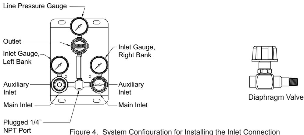
Figure 4. System Configuration for Installing the Inlet Connection
