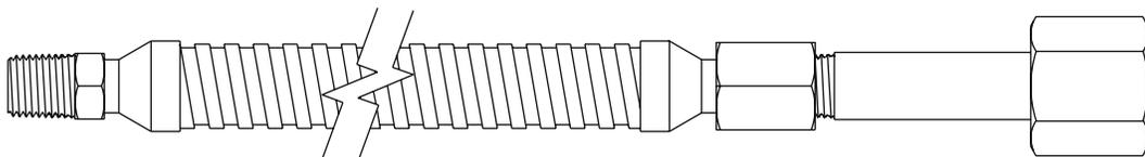
Figure 5. Pigtail with Cylinder Connection
