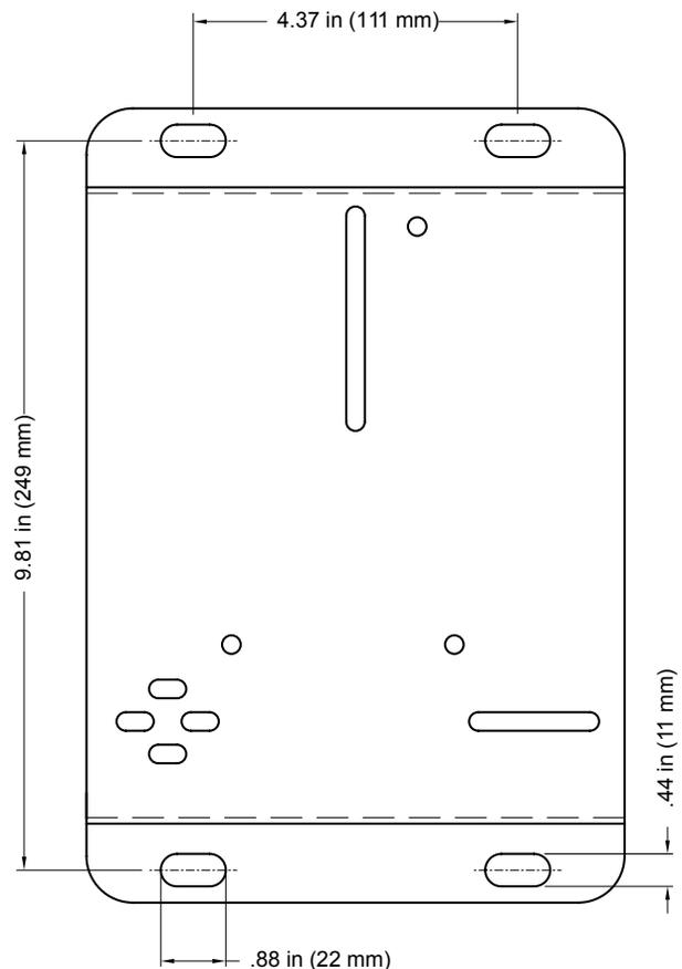
Figure 2 - Installation Bracket
