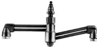
The Adjustable Duplex Tip Holder permits 2 parallel cuts to be made simultaneously with one CONCOA cutting torch. Easily adjusted to cut metal strips between 1 ¼" and 12 " wide (3.2 and 30.5 cm), it can be used for work to 3" (7.6 cm) plate thickness.
