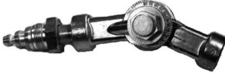
need to angle the torch. Total angular adjustment on either side of the vertical plane is 125°. The additional 35° from the horizontal enables cutting from below the work level when necessary. Indexing marks of 5° increments are forged in the face of the adapter body to facilitate adjustment at any required degree. Tip sizes up to number 6 can be used with this attachment.
