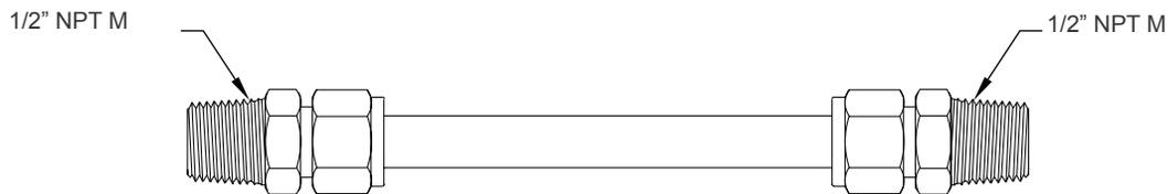
**Figure 7** - Manifold connector for the Maniflex system
