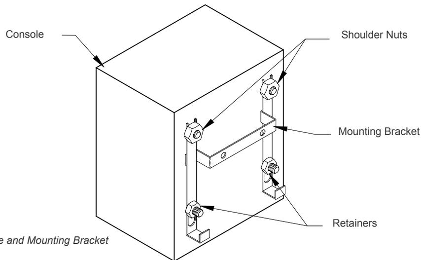
**Figure 5 - Console and Mounting Bracket**
