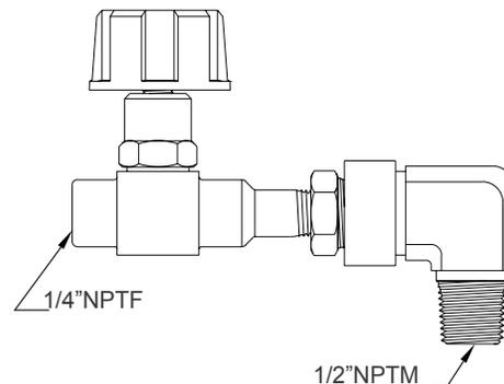
**Figure 9** - Diaphragm Valve with 1/2 inch NPT street elbow
