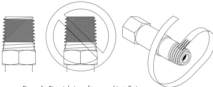
Figure 1 - Pictorial view of tape seal installation
