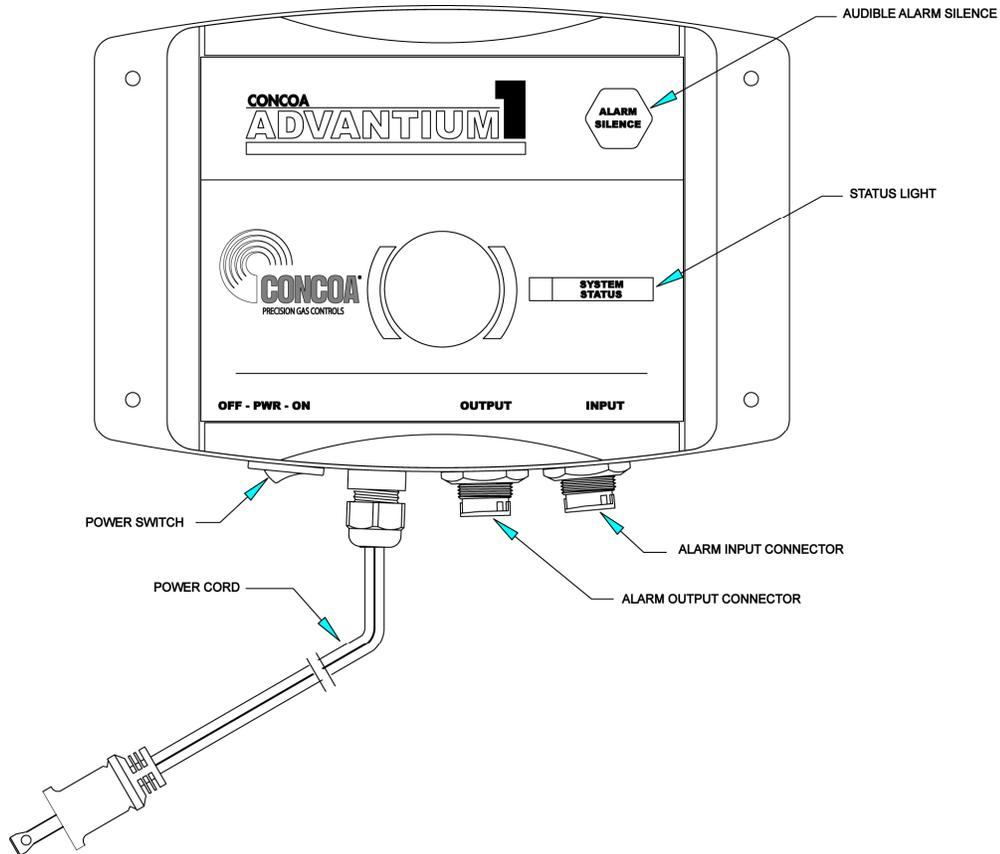
Figure 1 shows the location of the various inputs, outputs and indicators for the alarm. The Advantium 1 *Plus* is available in two models. The 5750011 is factory set to operate on 120VAC 50-60hz, The 5750012 is factory set to operate on 220VAC 50-60hz. **MAKE SURE THAT YOU HAVE THE CORRECT MODEL FOR THE SUPPLY VOLTAGE YOU WILL BE CONNECTING TO.**
