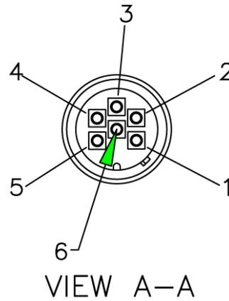
Using the pin assignments shown in Table 1 and the connector views in Figure 4 and Figure 5, solder the wires to the appropriate pins. After soldering is complete, slide the locking nut over the connector body. Snap the cable retainer into the body and then slide the protective cover over the cable retainer.
