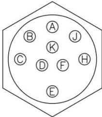
Looking at Connector On Back of Differential Pressure Switch (Appears mirror image on the connector on the cable assembly)
