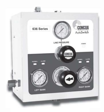
The 636 Series AutoSwitch provides a continuous supply of nonflammable industrial gases at a constant delivery pressure from two high pressure banks. Pressure switches enable visual alarms and an optional remote alarm to notify the user of the need to replenish a depleted bank.
