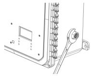
NPT connections require the use of PTFE tape on the threads to make a gas tight seal. On stainless steel connections, the thread sealant helps prevent the connections from galling together when tightening or loosening. CONCOA uses PTFE tape on all of its NPT connections.
