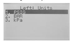
Use **Up** & **Down** buttons to highlight the desired units of measure.
