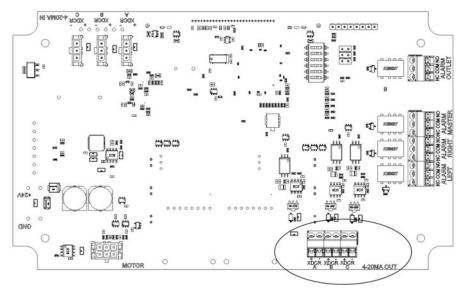
If connecting Left and Right 4-20 mA transducer outputs to an Altos 2, refer to the Altos 2 manual and the diagram to the right:
