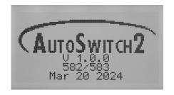
The about screen displays the system part number as well as the installed software version.
