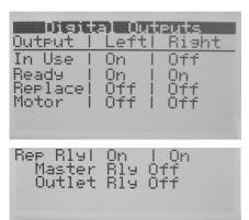
The unit displays all the digital outputs on this screen. Press the **Down** button to see additional outputs. A non-functional output can be checked here. For example, if the left relay should be active but is not closing its contact as expected, this screen will confirm if the system is trying to activate the contact (implying a bad relay) or not (something else is preventing the system from activating the relay like a higher priority status event).
