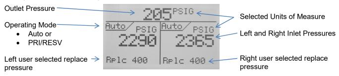
In the event of a major error, the LCD Main Screen will turn red and display the highest priority notification status. If in this state, the unit needs maintenance before normal operations can resume.
