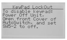
Keypad Lockout provides instructions for changing the Keypad Lockout mode. Default mode is OFF.
