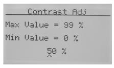
Contrast adjustment allows the screen contrast to be adjusted. Pressing the up or down buttons will increase or decrease the contrast ratio of the screen. The default factory value is 50. The value can be adjusted between 0 (the lightest) and 99 (the darkest). To save the selected ratio, press the right button.
