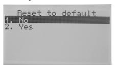
Activating Factory Reset restores all parameters to the factory default state and reboots the device.
