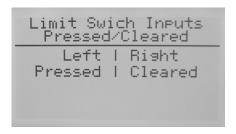
Digital Inputs lists the status of each of the motor limit switches, and shows if they are open or closed. This screen would help show the cause of a "Miswire" fault. Only one switch should be pressed at any given time, unless the unit is in the middle of a bank-select, in which case neither switch should be pressed.
