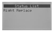
This example shows a right low pressure event, indicating the right cylinder needs replacement. If multiple status events are shown, the up/down buttons can scroll through them.
