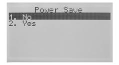
Power Save Mode, when enabled, turns off the LCD screen after fifteen minutes of inactivity (when the screen is off, the unit will still function as normal). Pressing any button on the front cover will wake up the LCD screen. Default mode is OFF
