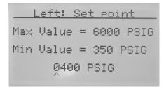
Max and Min values provide the limits for the replace set point.
