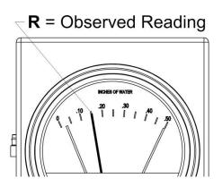
Dial the low set point pointer to "0", and then dial it back up to approximately half the observed vacuum reading.
