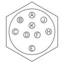
Looking at Connector On Back of Differential Pressure Switch (Appears mirror image on the connector on the cable assembly)
