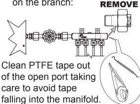
Clean PTFE tape off end of burst disk ass'y, and apply fresh tape.
