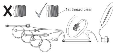
Fasten the extension tube to the existing manifold block, the extension block to the extension tube, and the burst disk ass'y to the extension block:
