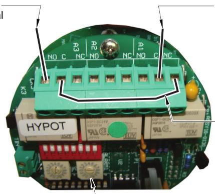
Connect A1 "C" to "+12 VDC" terminal of appropriate input on 585 1008.
