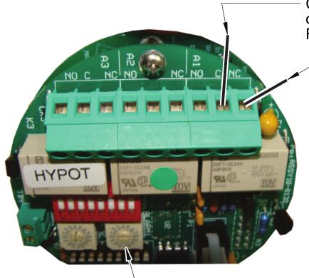
Connect A1 "C" to "+12 VDC" terminal of appropriate input on 585 1008. Refer to CONCOA ADI # 99065850.
