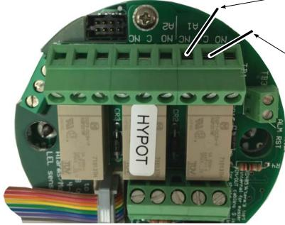
Connect A1 "NC" to "CONTACT" terminal of appropriate input on 585 1008. Refer to CONCOA ADI # 99065850.
