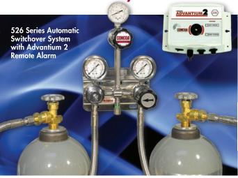
The automatic switchover systems provide continuous delivery for high purity, ultra high purity and corrosive gases. Typically used in the laboratory or process plant, the system automatically changes cylinder priority from a primary bank to a reserve bank without transmitting pressure fluctuations to the use line.
